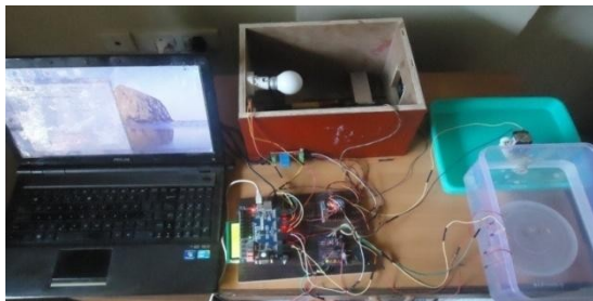
Fig.2. Experimental setup photograph for temperature, liquid level and humidity control
