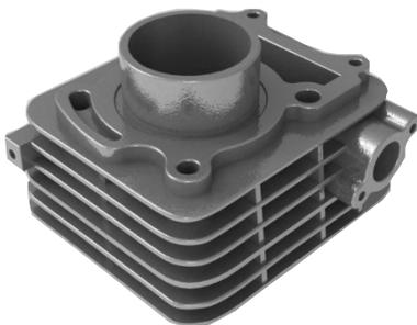
Fig. 11: CAD Model for TVS Wego Block
