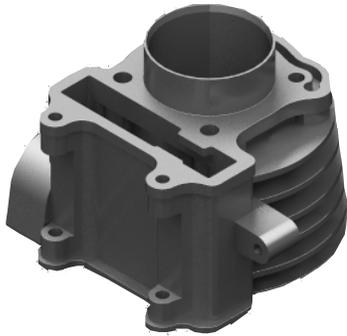
Fig. 1: CAD Model for Honda Activa Block
