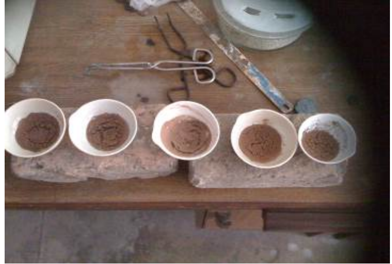
Figure 2: Thermal activation of source material at M_{700} , M_{650} , M_{600} , M_{400} , and M_{200} ( M = temperature, left to right).
