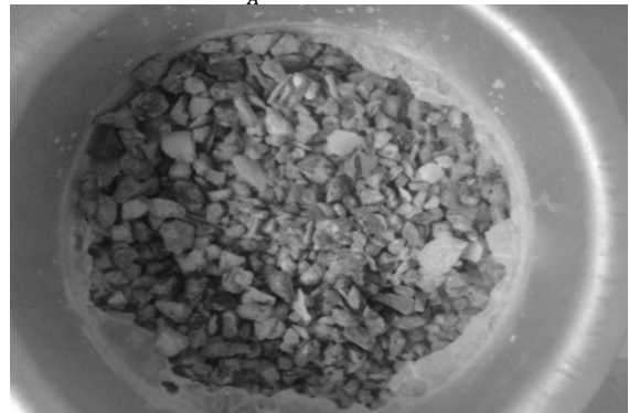
Fig 7 Sample after alternate heating and cooling for 5 days
