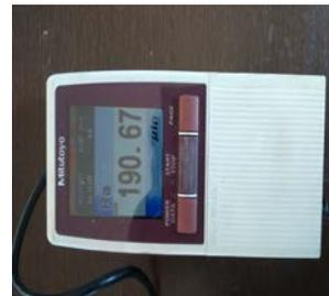
Fig. 6 Surface Roughness Tester
