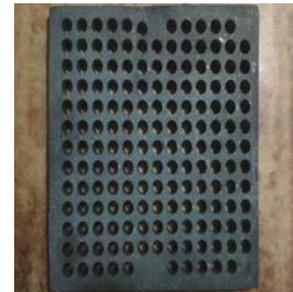
Fig. 5 SG Plate After Machining
