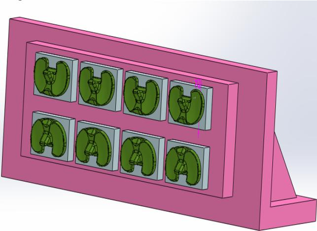
Figure 4: Angle Plate as Fixture for Operation II
