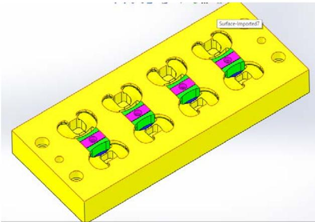
Figure 7: Assembly of Fixture with Wedge Clamp
