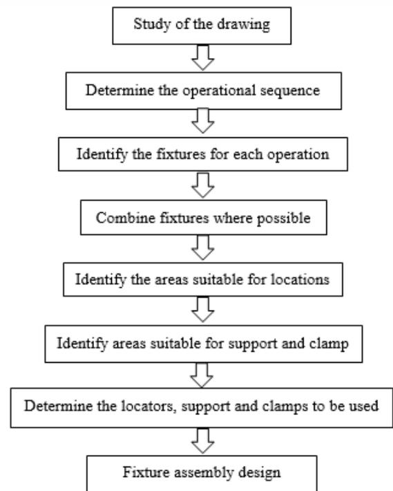
Figure 2 Flow Chart for Fixture Design
