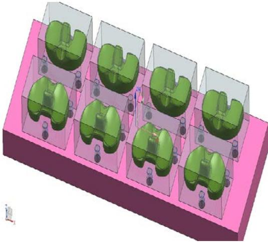
Figure 3: Base Plate as Fixture for Operation I
