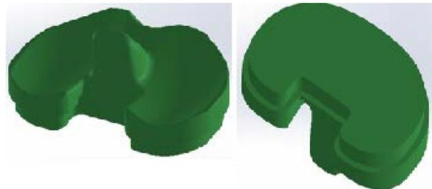
Figure 1: Top and Bottom View of Tibial Insert
