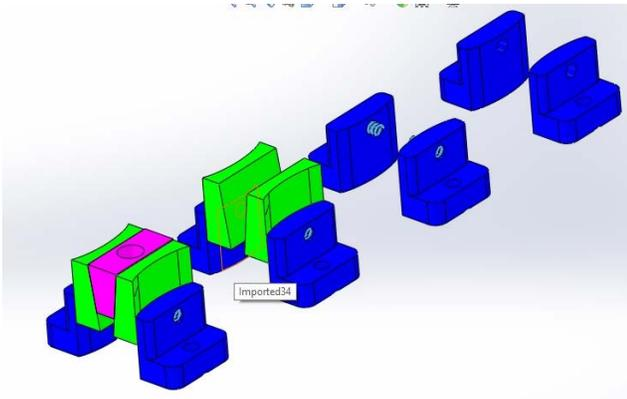
Figure 6: Elements of Wedge Clamp
