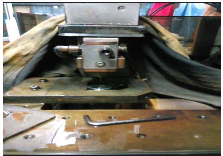
Fig.3.2: Working zone of Wire electrical discharge machining
