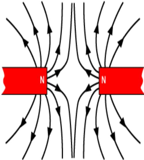
Fig 2.1: Repulsive force diagram between two same poles of two magnets
