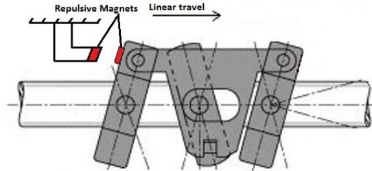
3.2: Position of magnets and end stop after reversal of bearings
