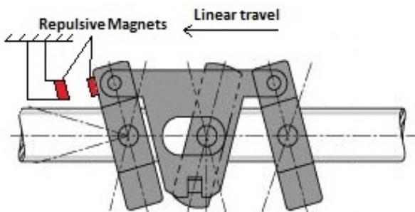
Fig 3.1: Position of magnets and end stop before reversal of bearings
