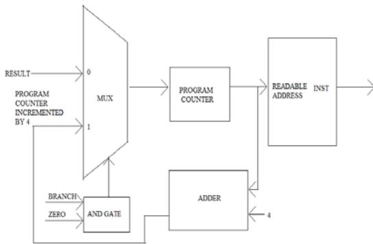
Fig. 1: Block diagram of instruction fetch unit
