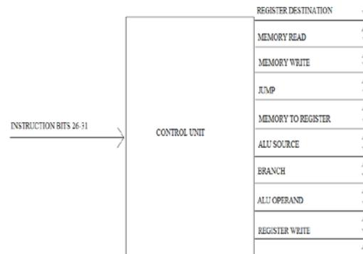
Fig. 4: Block diagram of control unit
