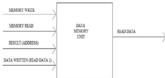
Fig.6: Block diagram of data memory unit
