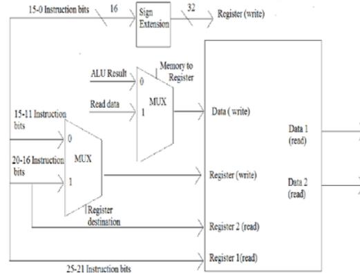
Fig. 3: Block diagram of instruction decode unit
