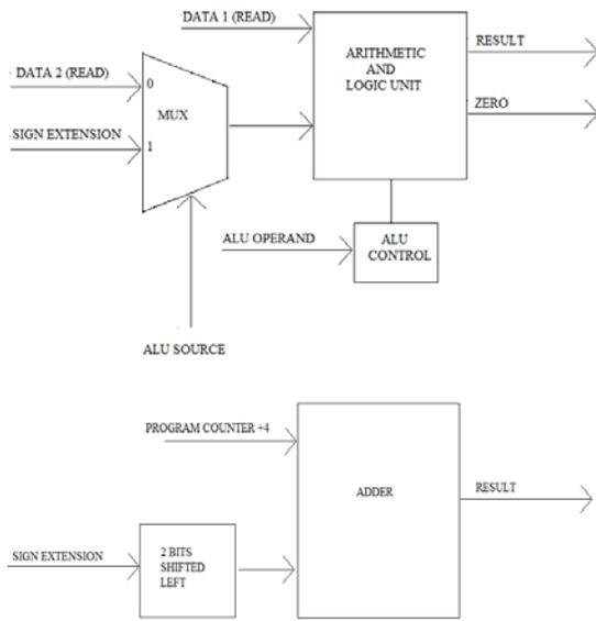
Fig.5: Block diagram of execution unit
