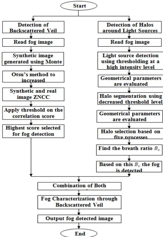
Fig 5.6: Flow diagram of proposed system
