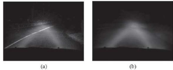
Fig. 4 (a) The actual image grabbed while driving. (b)The image obtained after applying the Rank Filter (median).
