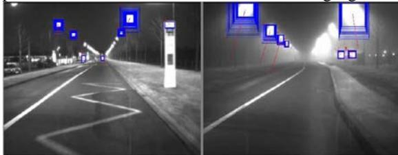
Fig. 6 (a) The street lights without fog seems to be different component. (b) The detection of potential source in the presence of fog seems to be as connected component.
