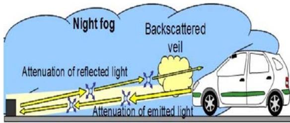
Fig. 2 The effect of Backscattered veil due to the formation of night fog
