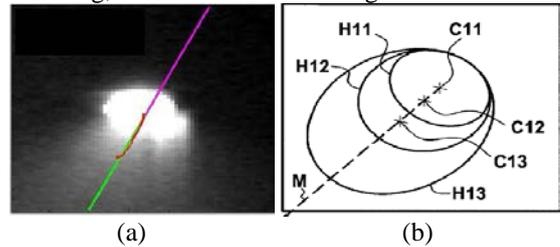
Fig.7 (a) The calculation of intensity of light along its direction. (b) This is the geometrical representation of how intensity of light is calculated and how the threshold is determined where H represents Halo and C represents Center of Gravity (COG).
