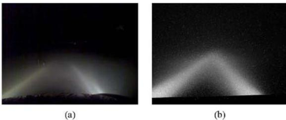
Fig. 3 (a) The actual captured image in Fog and (b) The synthetic image captured using Monte-Carlo ray tracing Software.
