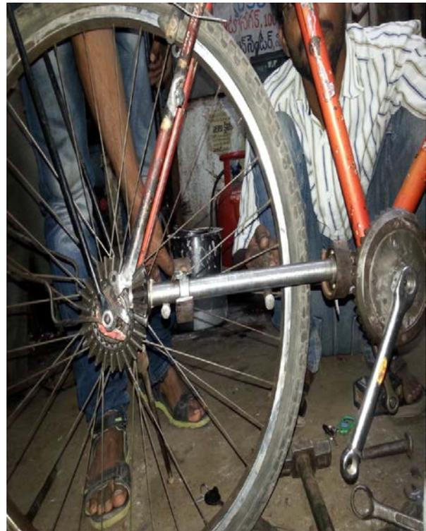
**Figure-9.** Assembly of Shaft drive mechanism to bicycle
