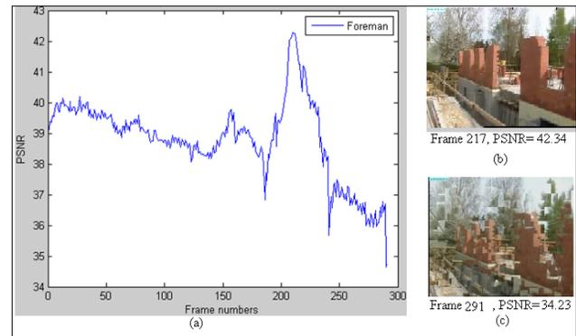
Figure.4: (a) PSNR vs. Frame numbers; (b) and (c) show frames with different quality values of Foreman video clip.
