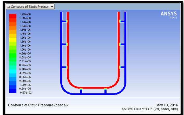
Fig 3.2.4. Contours of static pressure for Tri-chloro ethylene glycol
