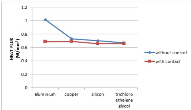
**Graph 3.5.5.** Annular bend tube without and with contact Heat flux comparison graph
