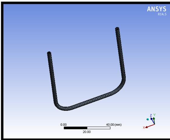
Fig 3.3.8. 3DAnnular bend tube meshed model
