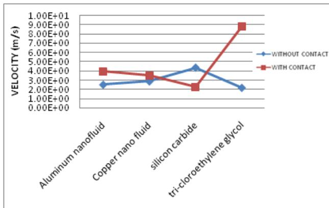
**Graph 3.5.2.** Annular bend tube without and with contact velocity comparison graph
