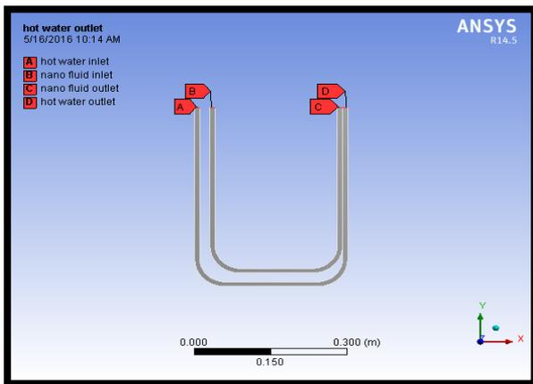
Fig 3.2.9. Annular bend tube inlet & outlet named model
