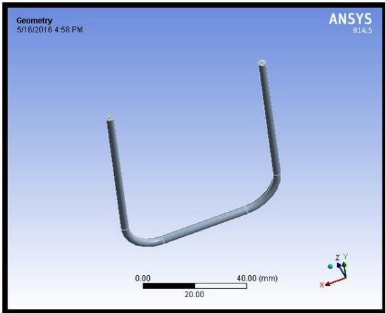
Fig 3.3.7. 3DAnnular bend tube imported model to ANSYS
