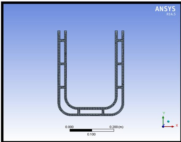
Fig 3.2.2. Annular bend tube meshed model
