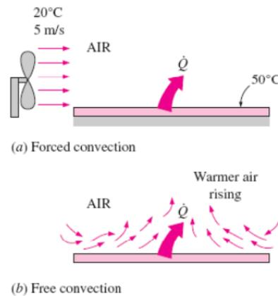
Fig 1.1. Forced Convection and Free Convection
