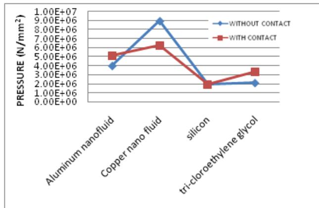
**Graph 3.5.1.** Annular bend tube without and with contact pressure comparison graph
