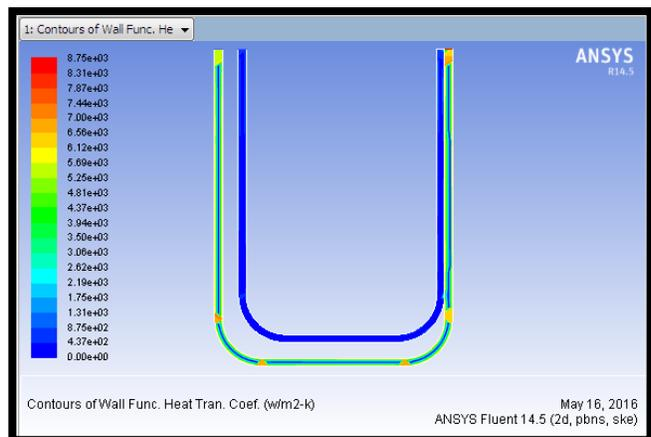
Fig 3.2.12. Contours of Heat transfer coefficient for Tri-chloro ethylene glycol
