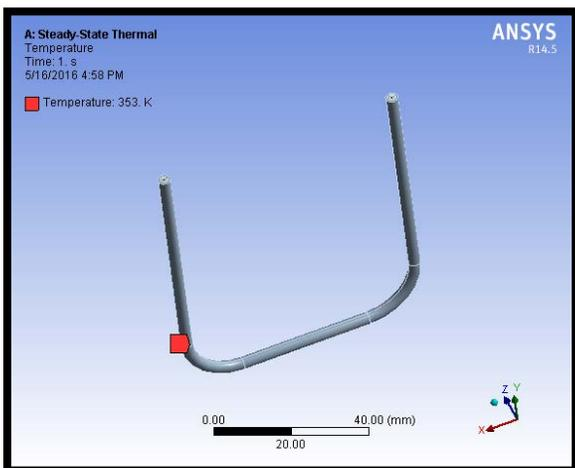
Fig 3.3.9. 3DAnnular bend tube with applied temperature
