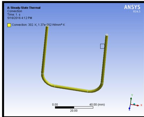
Fig 3.3.4. 3D Annular bend tube with applied convection
