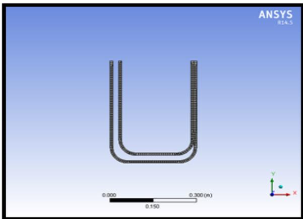
Fig 3.2.8. Annular bend tube meshed model
