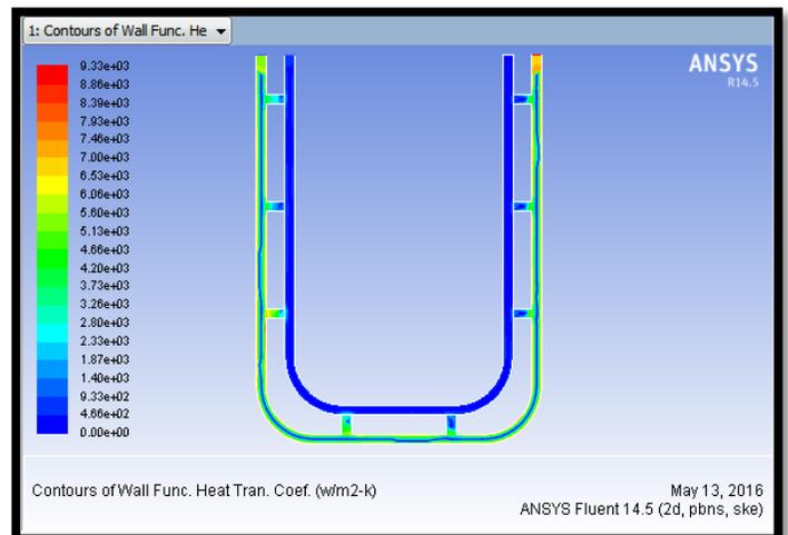
Fig 3.2.6. Contours of Heat transfer coefficient for Tri-chloro ethylene glycol
