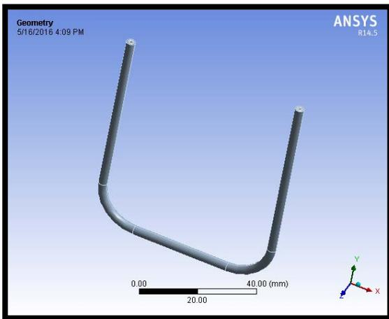
Fig 3.3.1. 3D Annular bend tube imported model to ANSYS
