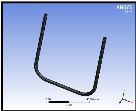
Fig 3.3.2. 3D Annular bend tube meshed model
