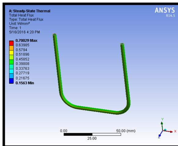
Fig 3.3.6. Results of Heat flux
