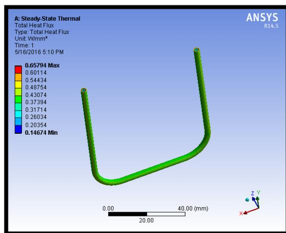
Fig 3.3.12. Results of Heat flux
