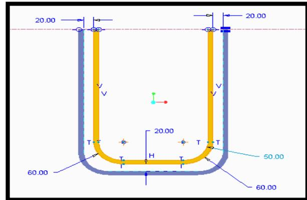
Fig 3.1.1 Annular bend tube 2D model with dimensions
