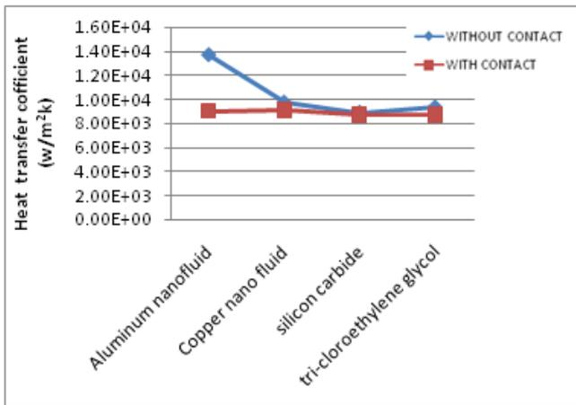
**Graph 3.5.3.** Annular bend tube without and with contact Heat transfer coefficient comparison graph
