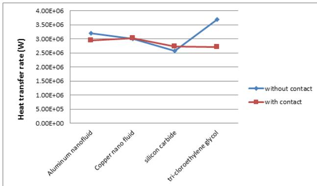
**Graph 3.5.4.** Annular bend tube without and with contact Heat transfer rate comparison graph
