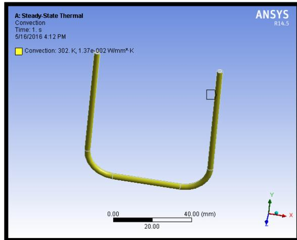
Fig 3.3.10. 3DAnnular bend tube with applied convection
