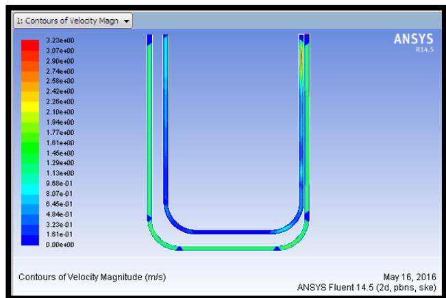
Fig 3.2.11. Contours of Velocity for Tri-chloro ethylene glycol
