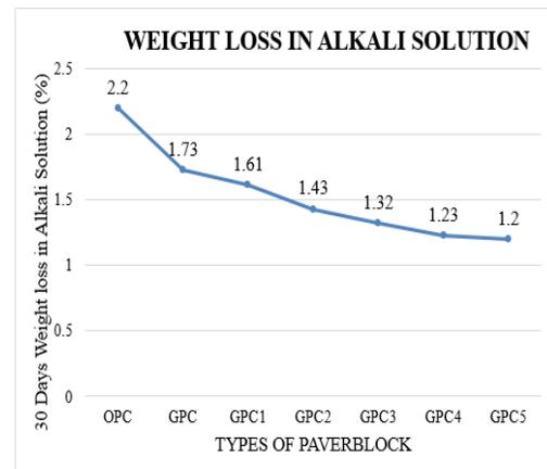
Fig. 7. weight loss in alkali solution variation of mixes
