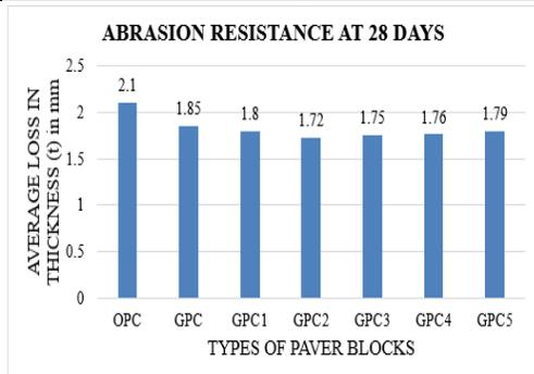
Fig. 2.. Abrasion resistance at 28 days
