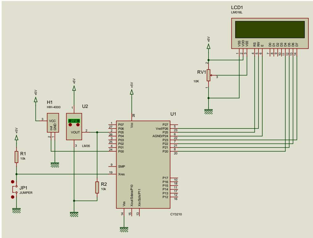
Figure 1: System Schematics
