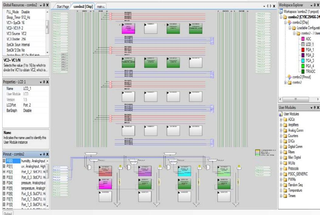
Figure 2: PSoC configuration window
