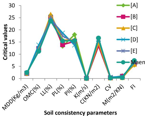
Figure 2; Mechanical behaviour of soil within the dumpsites.
