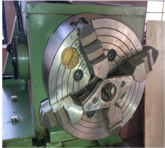
Fig .2 preparation of Convergent- Divergent Nozzle manifold flange
