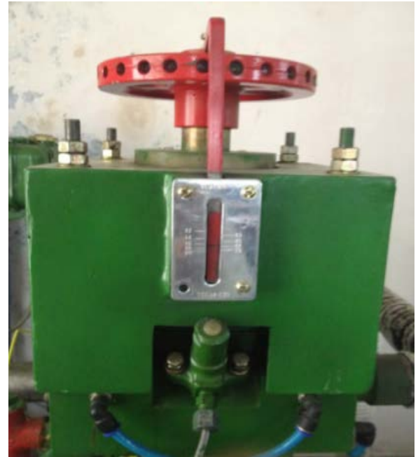
Fig.5 Variable compression ratio in diesel engine
