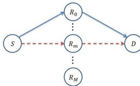
Fig. 1 System model for dual-hop relay communication systems.
