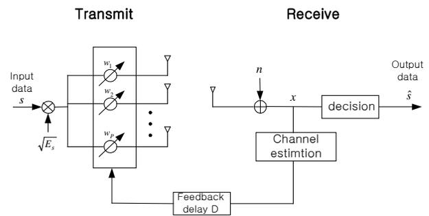
Fig. 1 Block diagram of a closed-loop TAD communication system.
