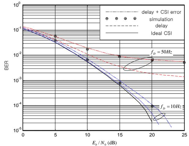
Fig. 3 Average bit error rate for  $f_D = 10$  Hz and 50 Hz ( $P = 2, d = 4, d/L = 20$ ).
