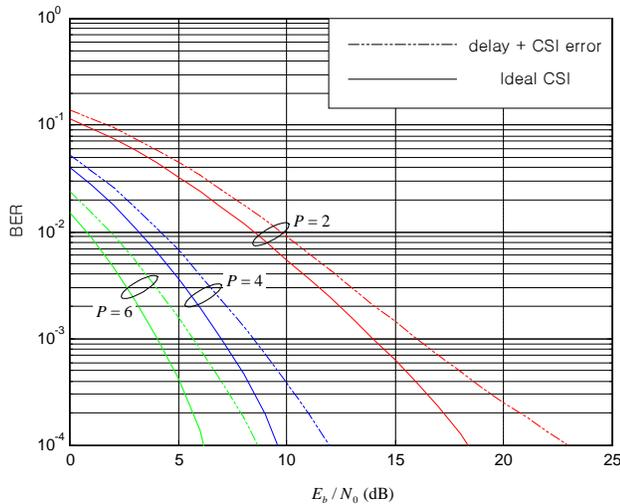
Fig. 4 BER versus the number of transmit antennas for  $f_D = 30$  Hz ( $d = P$ ,  $d/L = 20\%$ ).
