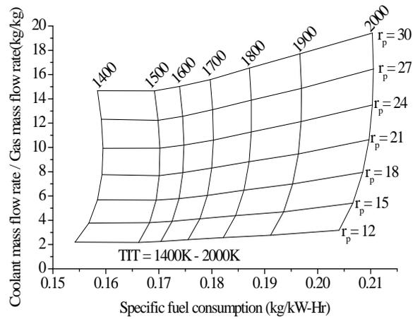
**Fig. 3.4** Variation of coolant requirement with SFC for SIBGT using AICC
