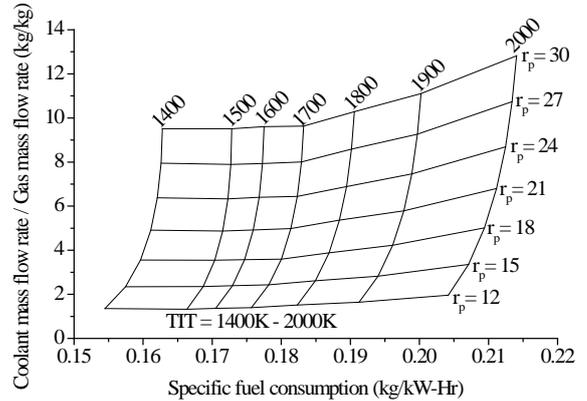
**Fig. 3.5** Variation of coolant requirement with SFC for SIBGT using AFC
