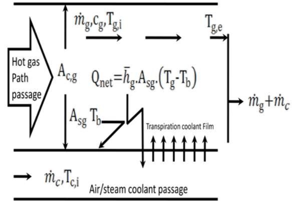
**Figure 2.4 Model for transpiration cooling of turbine blade**
