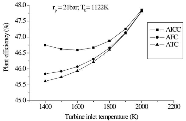
**Fig. 3.11** Variation of plant efficiency with TIT for SIBGT using AICC, AFC and ATC
