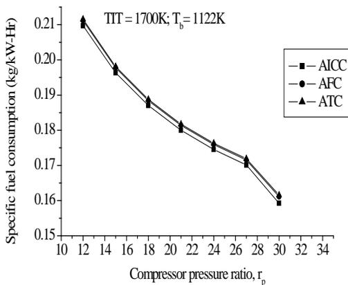
**Fig. 3.9** Variation of specific fuel consumption with  $r_p$  for SIBGT using AICC, AFC and ATC
