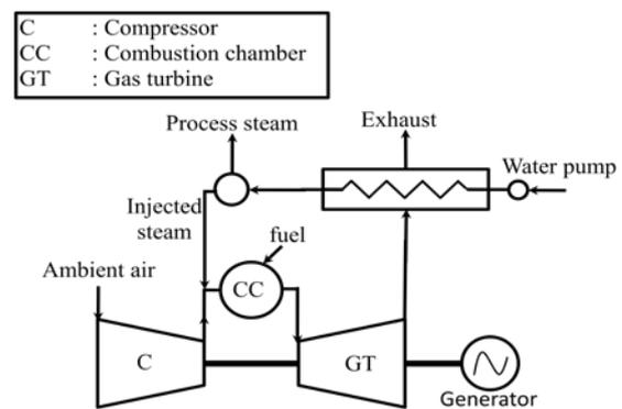
**Figure 1.1 Schematic diagram of a Steam Injected Gas Turbine Cycle**
