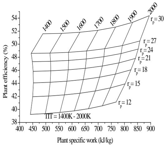
**Fig. 3.1** Variation of plant efficiency with plant specific work for SIBGT using AFC
