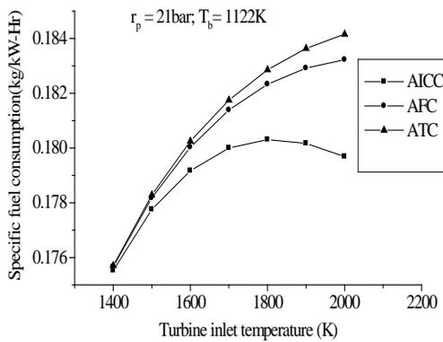
**Fig. 3.13** Variation of SFC with TIT for SIBGT using AICC, AFC and ATC
