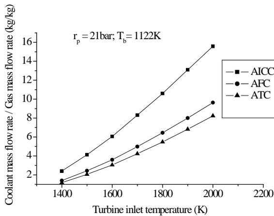
**Fig. 3.14** Variation of coolant requirement with TIT for SIBGT using AICC, AFC and ATC
