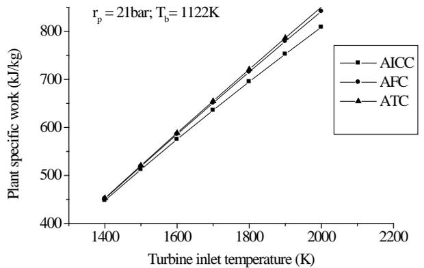
**Fig. 3.12** Variation of plant specific work with TIT for SIBGT using AICC, AFC and ATC
