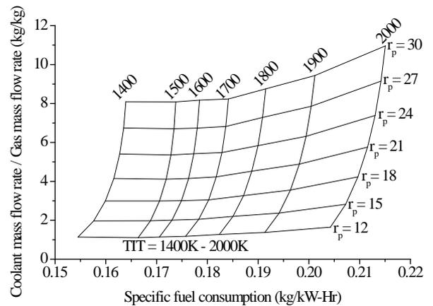
**Fig. 3.6** Variation of coolant requirement with SFC for SIBGT using ATC
