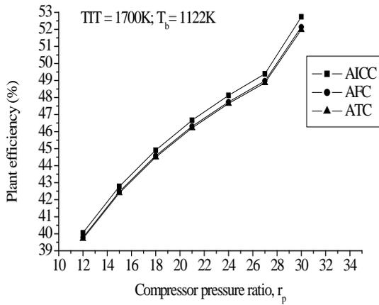
**Fig. 3.7** Variation of plant efficiency with  $r_p$  for SIBGT using AICC, AFC and ATC
