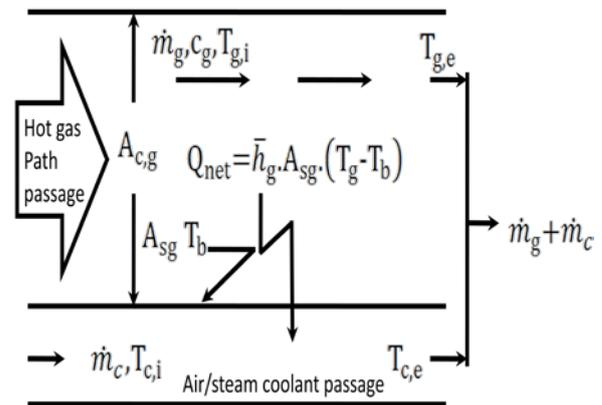
**Figure 2.2 Model for open loop internal convection turbine blade cooling**
