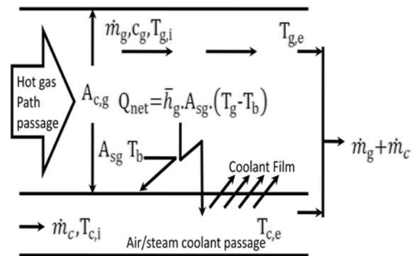
**Figure 2.3 Model for open loop film cooling of turbine blade**
