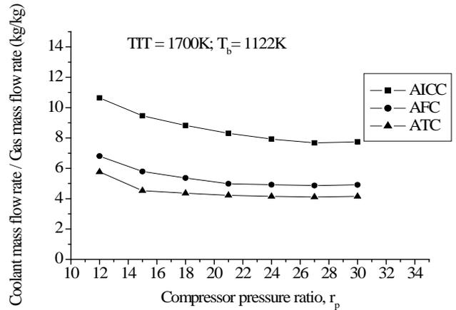
**Fig. 3.10** Variation of coolant requirement with  $r_p$  for SIBGT using AICC, AFC and ATC
