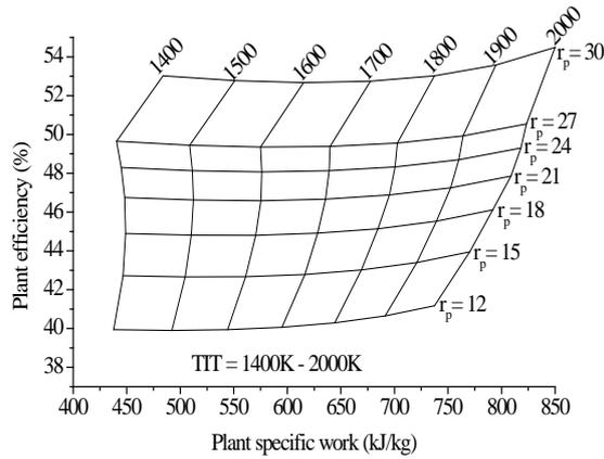
**Fig. 3.2** Variation of plant efficiency with plant specific work for SIBGT using AICC
