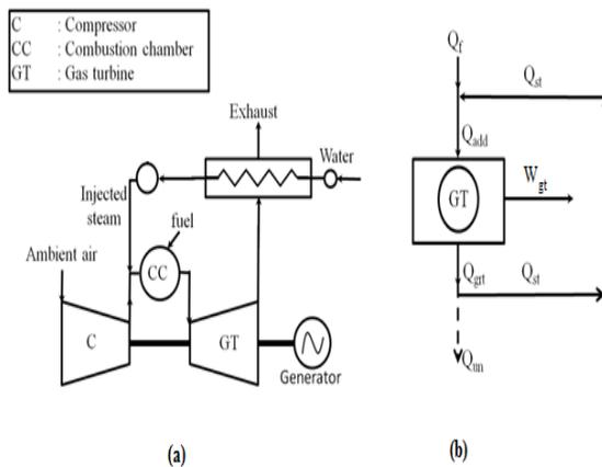
**Figure 1.2 (a) Schematic diagram of a mixed cycle power plant (b) Energy flow diagram of mixed cycle power plant**
