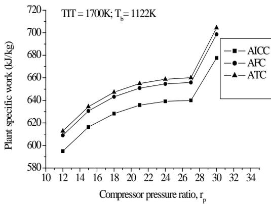
**Fig. 3.8** Variation of plant specific work with  $r_p$  for SIBGT using AICC, AFC and ATC
