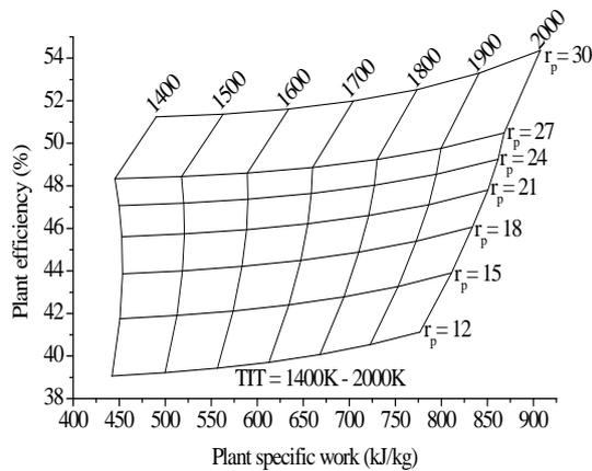
**Fig. 3.3** Variation of plant efficiency with plant specific work for SIBGT using ATC
