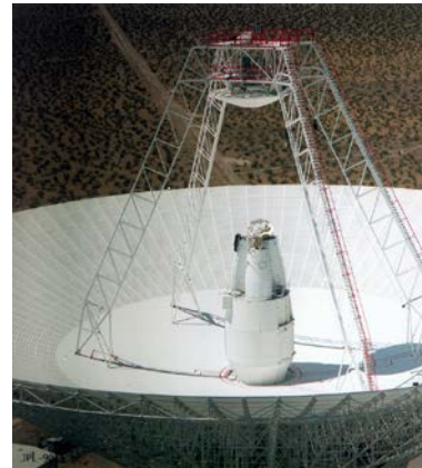
Fig. 1. Photo of a Cassegrain antenna used for spacecraft communications, located in Canberra, Australia [1].
