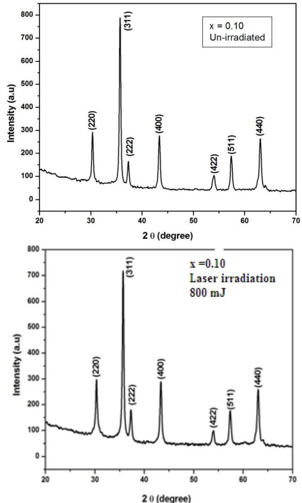
Fig. 2. XRD pattern of Un-irradiated and laser irradiated  $\text{Ni}_{1.1}\text{Zr}_{0.1}\text{Fe}_{1.8}\text{O}_4$  nanoparticles
