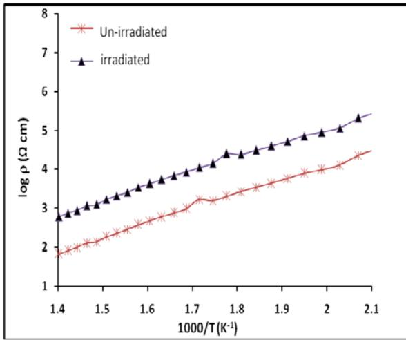
Fig. 3. Variation of DC electrical resistivity with reciprocal of temperature for Un-irradiation  $Ni_{1.1}Zr_{0.1}Fe_{1.8}O_4$  nanoparticles
