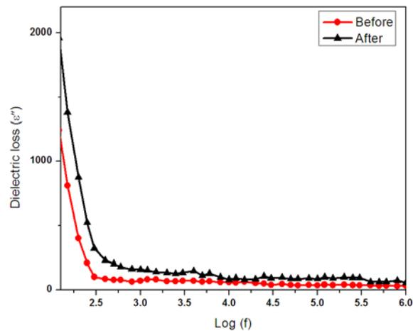
Fig. 4 (b) Variation of the dielectric loss ( $\epsilon''$ ) with frequency log (f) for un-irradiation and (1200 mJ dose rate) Nd: YAG laser irradiation
