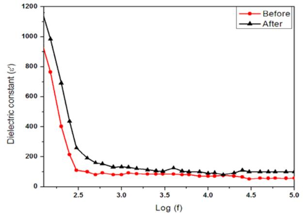
Fig. 4 (a) Variation of the dielectric constant with frequency log (f) for un-irradiation and (1200 mJ dose rate) Nd: YAG laser irradiation
