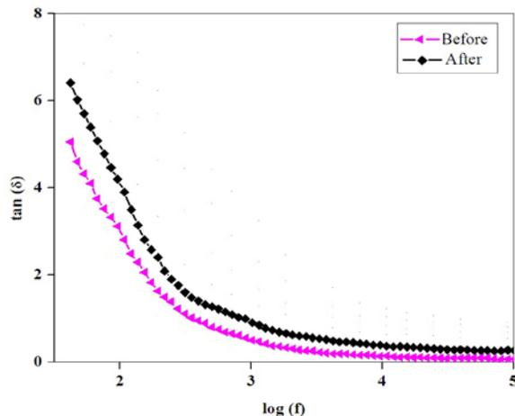
Fig. 4 (c) Variation of the tangent loss ( $\tan\delta$ ) with frequency  $\log(f)$  for un-irradiation and (1200 mJ dose rate) Nd: YAG laser irradiation  $\text{Ni}_{1.1}\text{Zr}_{0.1}\text{Fe}_{1.8}\text{O}_4$  nanoparticles
