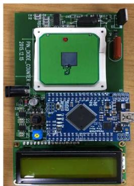
Fig. 2 Implemented PIN photodiode radon counter
