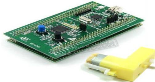
Fig. 3 Operation part (STM32f051 - Motor).
