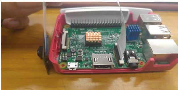
Fig. 2 The sensor part (Raspberry pi 2).
