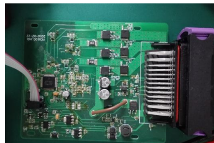
Fig. 11 the controller of the fan
