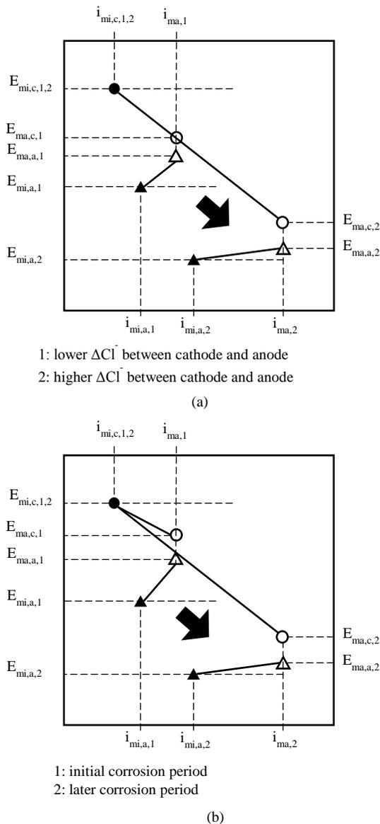
**Fig. 10** Corrosion mechanism in chloride-induced macro-cell corrosion
