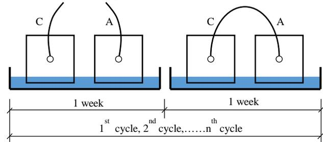
**Fig. 4** The cycle process of experiment
