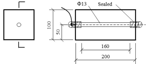
Fig. 3 Cathode and Anode specimen
