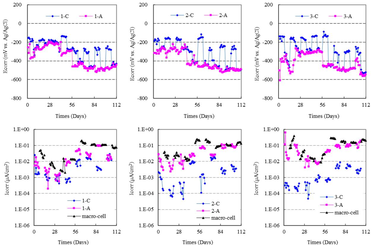
**Fig. 5** Time evaluation curve of half-cell potential, micro-cell current density, macro-cell current density in each case
