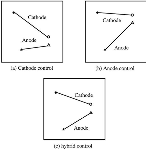
Fig. 2 Control mode of Macro-cell corrosion
