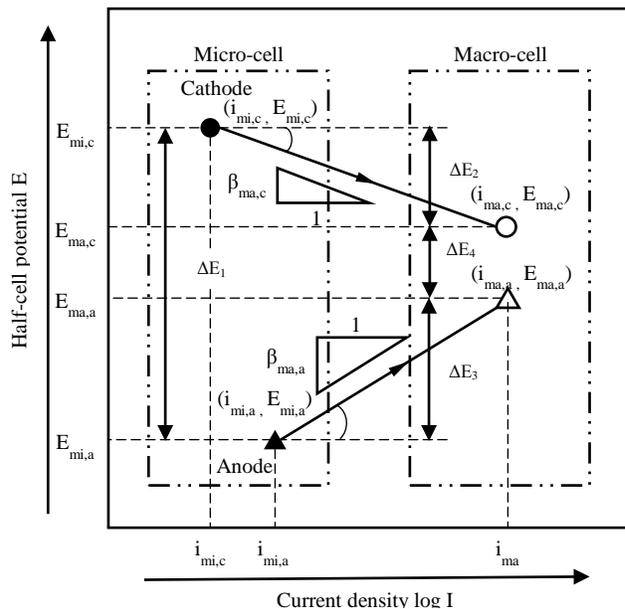
Fig. 1 Macro-cell corrosion model
