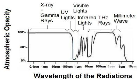
Fig 1. Atmospheric opacity of different cosmic radiations [4]
