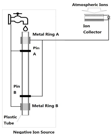
Fig . 4. Schematic view illustrating the prototype modeling the whole atmospheric ions collecting system
