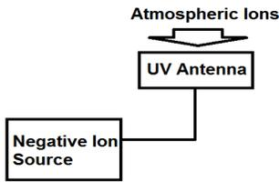
Fig. 2 Building Blocks of the Proposed Atmospheric Ion Collecting System
