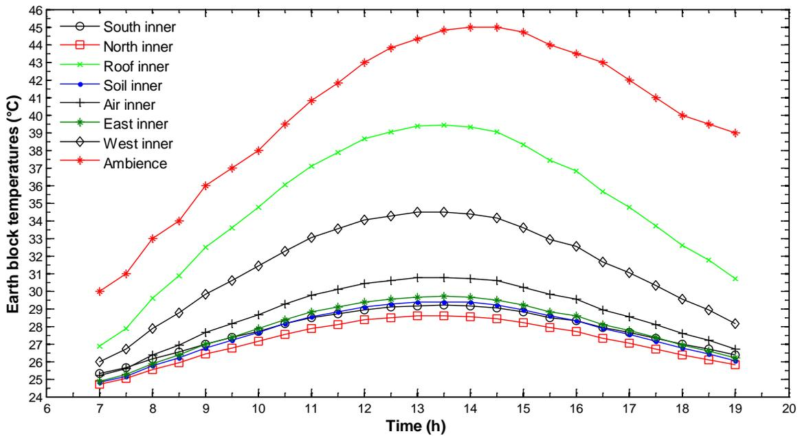
Fig. 8 Evolution profile of the temperature in the earth block building
