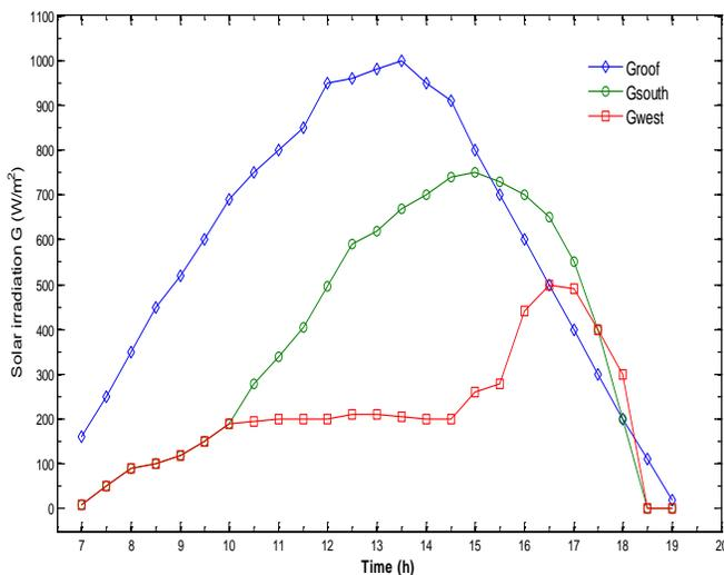
Fig. 3 Solar irradiation on different walls in June [4]
