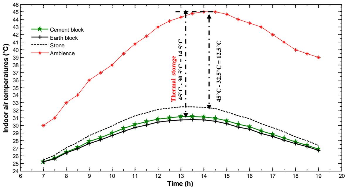
Fig. 11 Comparison of the temperatures of the indoor air of the buildings
