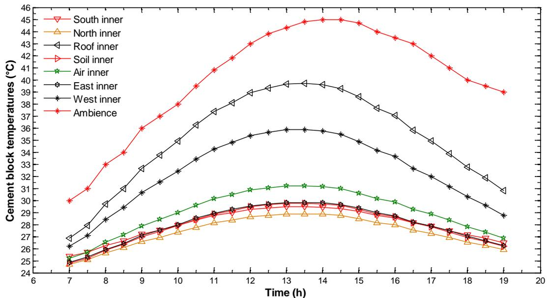
Fig. 7 Evolution profile of the temperature in cement block building
