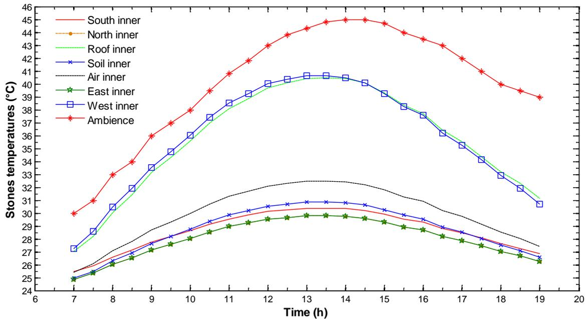
Fig. 6 Evolution profile of the temperature in stone building
