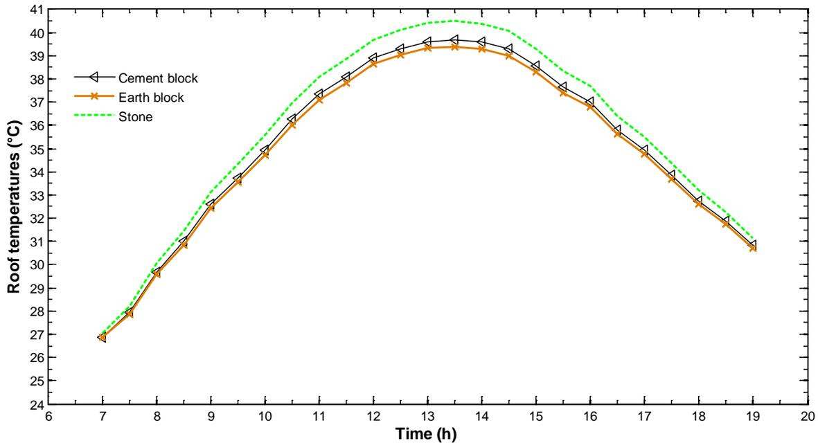
Fig. 10 Evolution profile of the temperature of the roof
