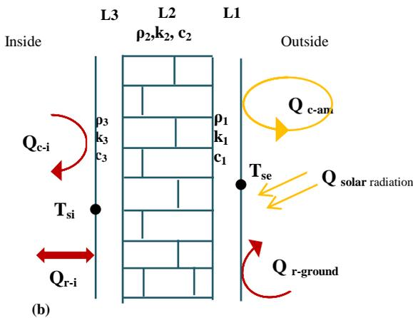
Fig.2 a) Wall's orientation and b) Definition sketch of a composite wall.
