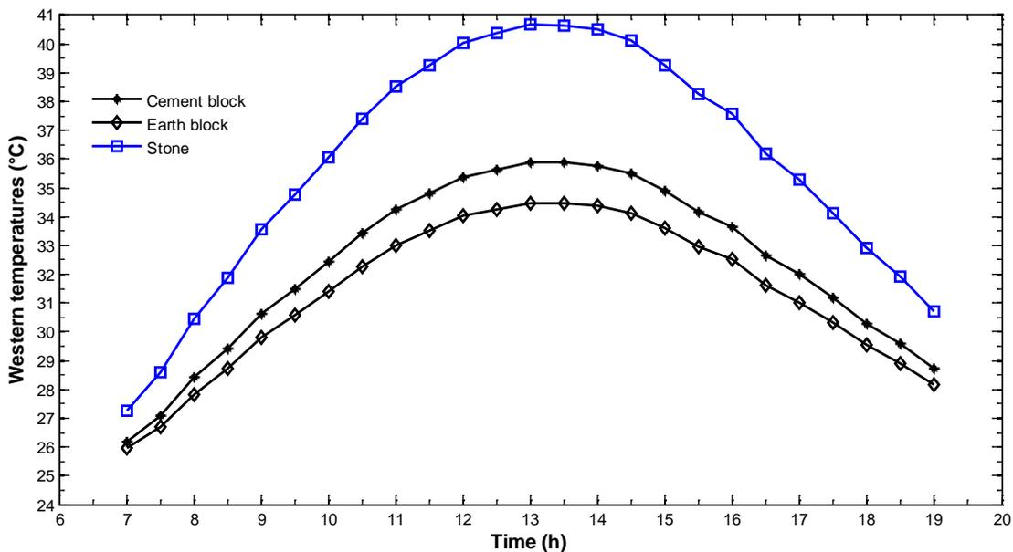
Fig. 9 Comparison of the temperatures of the western wall of the buildings
