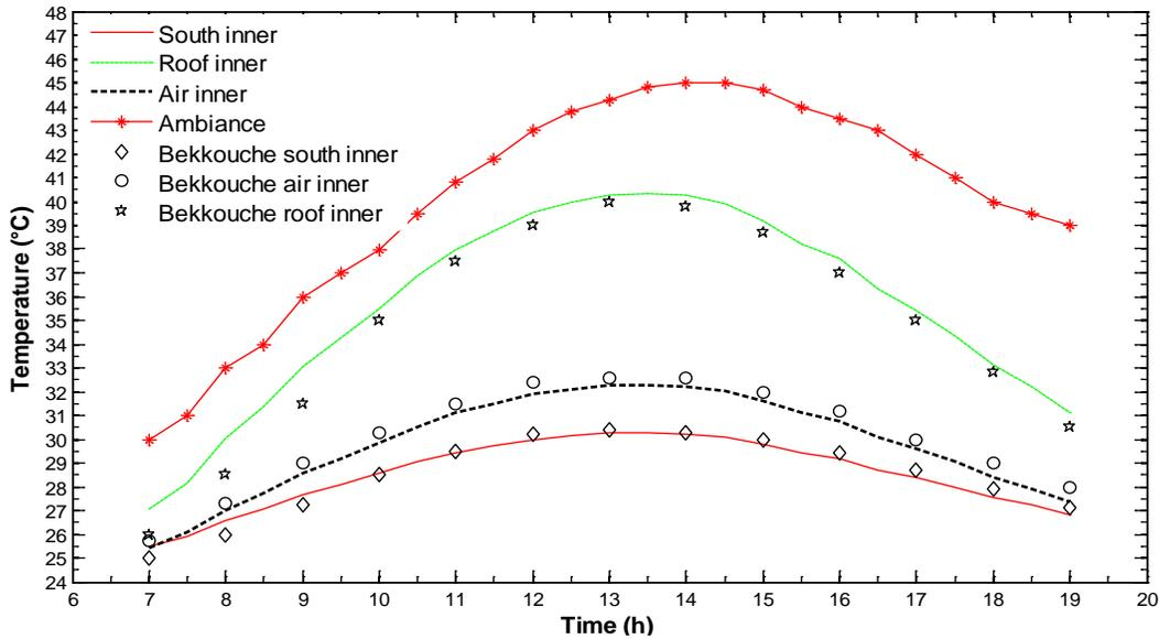
Fig. 4 Comparison between the external ambient temperature and inner temperatures of the building using stones ( $\rho=2580\text{kg/m}^3$ ;  $\lambda=2.8\text{W/mK}$ )
