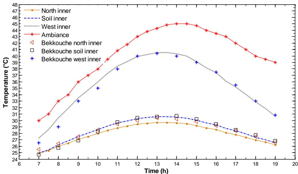
Fig. 5 Comparison between the external ambient temperature and inner temperatures of the building using stones ( $\rho=2580\text{kg/m}^3$ ;  $\lambda=2.8\text{W/mK}$ )
