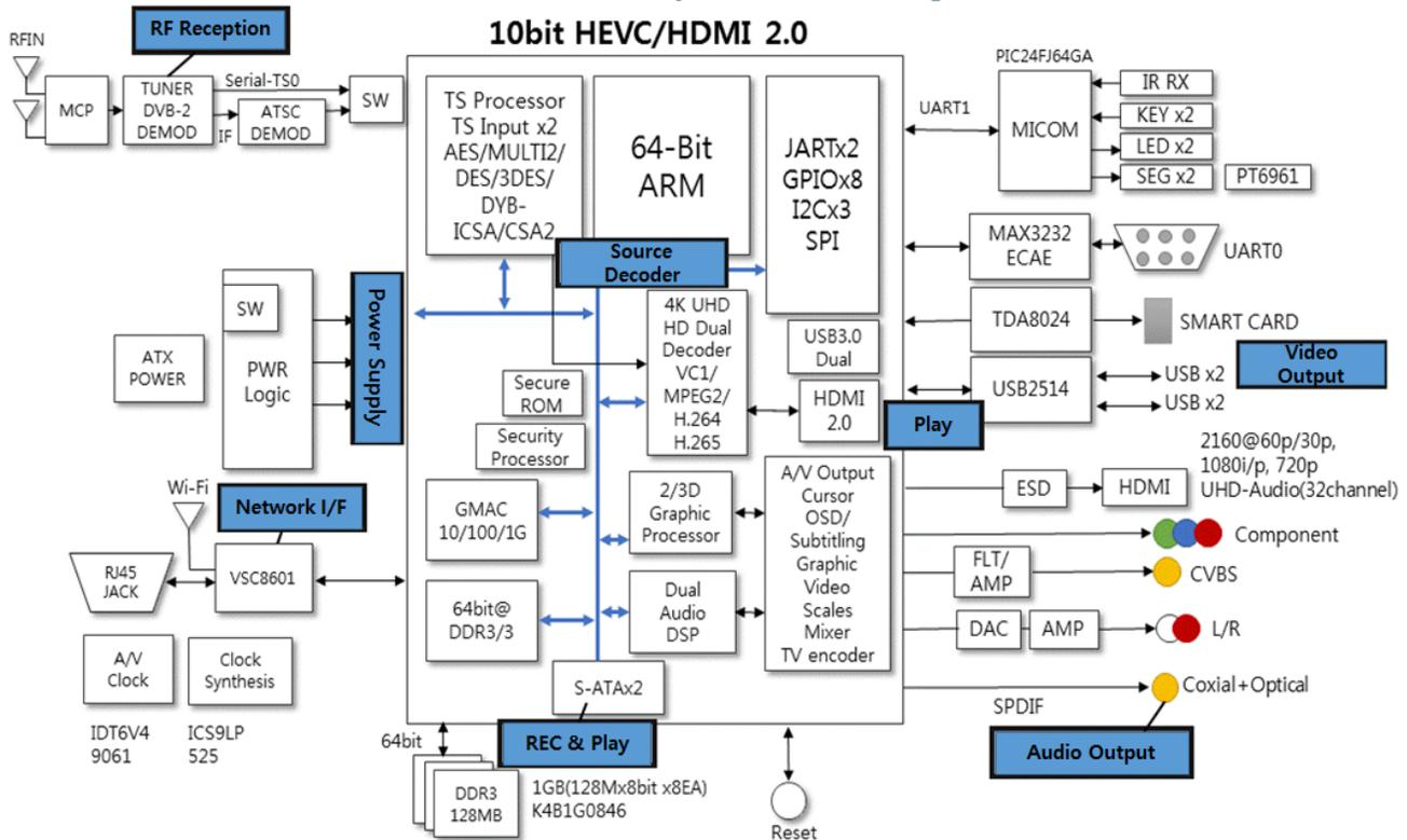
Fig. 2 Dual-mode (ATSC3.0/DVB-T2) set-top box block diagram
