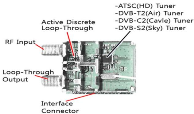
Fig. 3 Tuner of the RF signal reception block
