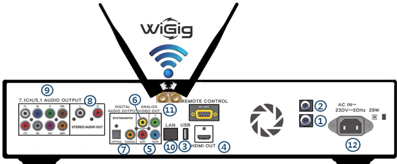
⑨ Analog multioutput - analog 5.1/7.1 audio output
