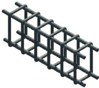
Fig 3. Reinforcement for R.C.C beams
