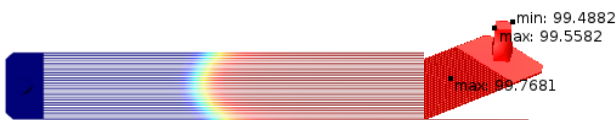
Figure 9. The location of full evaporation of the water in case t_5 = 60^\circ\text{C}
