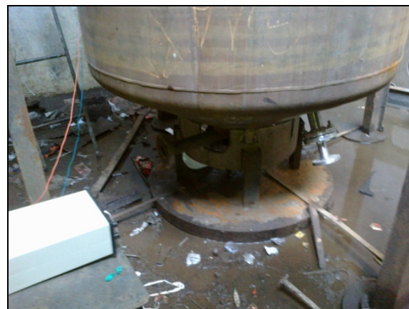
Fig. 11 Strain measurement with pressure vessel.
