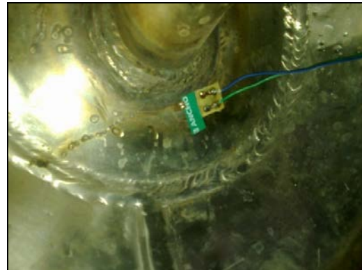
Fig. 10 Electrical strain gauge on shell.
