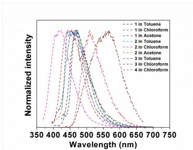
Fig.4. Emission spectra of boron compounds 1-4 in different solutions.
