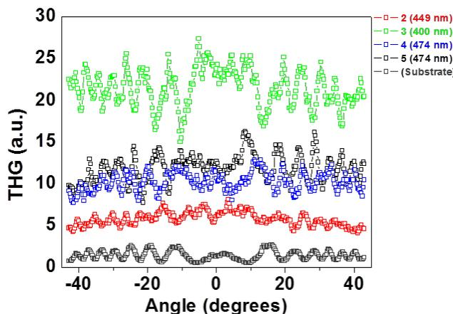
Fig. 5. THG Maker-fringe patterns for thin solids film doped with 30 wt% of compounds 2-4 and 5 for a 1-mm thick substrate without a film deposited on it. The fundamental wavelength is 1300 nm.
