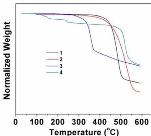
Fig. 7. TGA thermograms of boron compounds 1-4.
