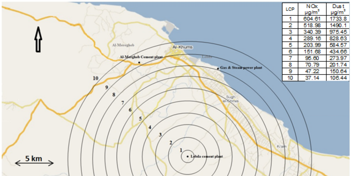
Figure 3. Concentration distribution of pollutants emitted from the Lebda Cement Plant (LCP) based on annual average wind speeds.
