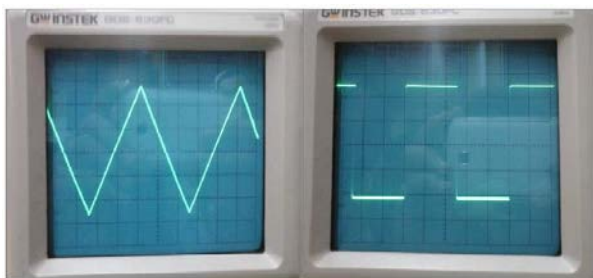
Fig.8. Waveform output from the Mobile phone based TENS
