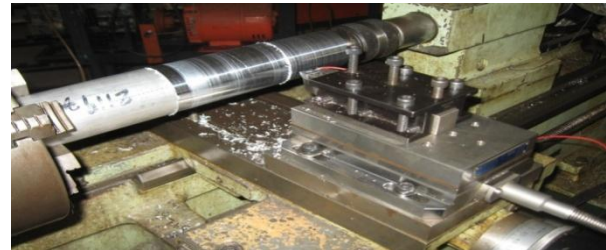
Fig 4.1 Kistler three components Dynamometer fitted with tool holder
