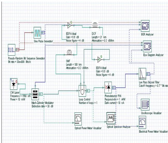
Fig. 1 Schematic for Post Compensation Scheme
