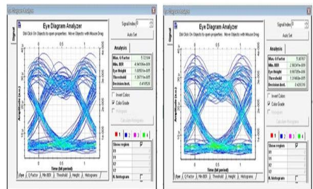
Fig 2: Eye diagrams at different frequencies
