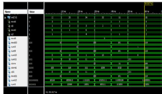
Fig.8: Simulation waveform for Test Code Generator and RQCG1.
