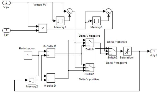
Figure 8(i) Perturb and Observe Algorithm simulation [35]
