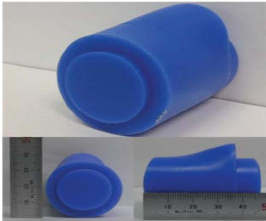
Fig.15 Curved surface machined using our developed system
