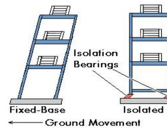
Fig. 3 Seismic behavior of building mounted without and with isolator.
