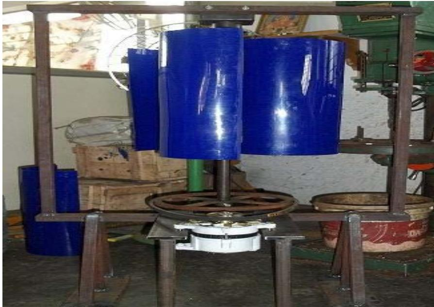
Fig 3.1 Fabrication of a Vertical Axis Wind Turbine
