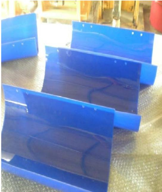
Fig.3.2 Rotor blades (acrylic material)
