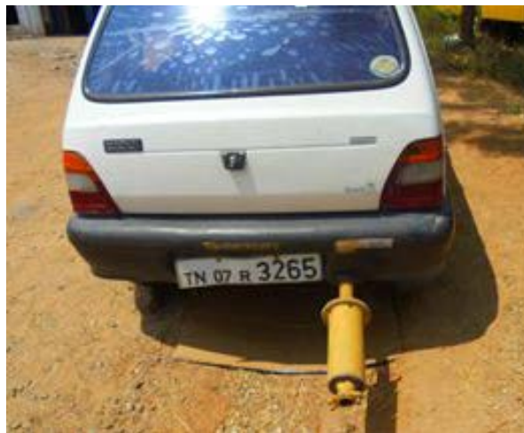
Fig. 6 CO 2 reduction catalyst assemblyat the tail pipe
