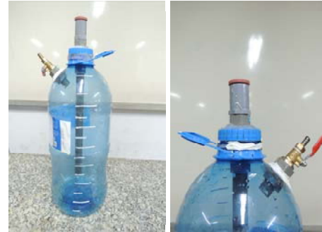
Fig 2 One-stage semi-continuous anaerobic digestion reactor.
