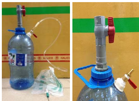
Fig 1 One-stage batch anaerobic digestion reactor.
