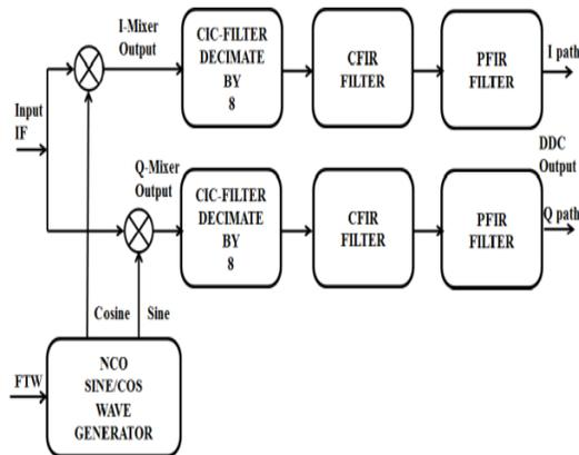
Fig. 1 Block Diagram of DDC
