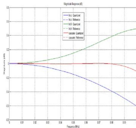
Fig. 7 Pass band details for the magnitude response of CIC filter and CFIR filter overlaid, along with the combined response of the 2
