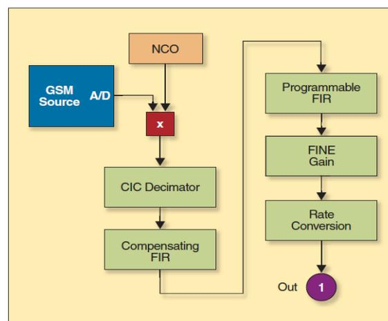
Fig. 4 GSM Digital Down Converter
