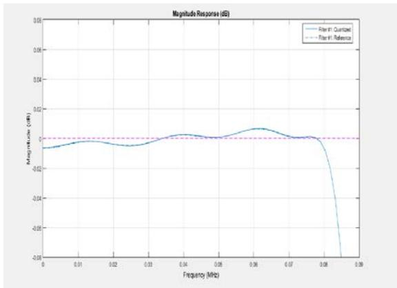
Fig. 9 Peak to Peak ripple less than 0.1dB
