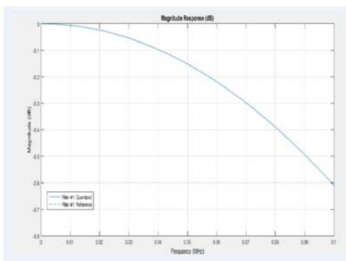
Fig. 6 Pass band details of scaled 5-stage CIC decimator
