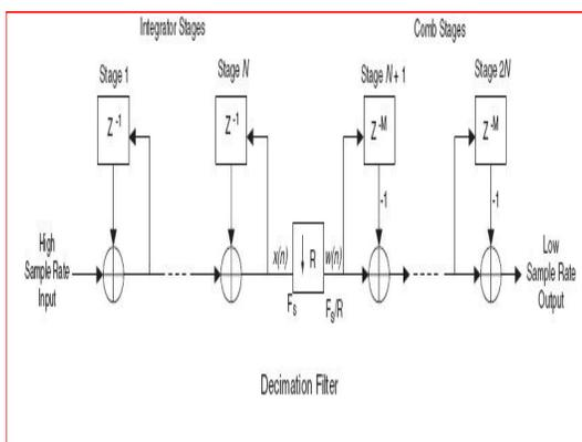
Fig. 3 CIC Filter structure
