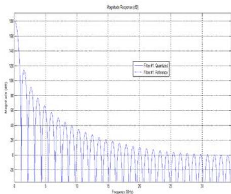
Fig. 5 Magnitude Response of 5 Stage CIC filter
