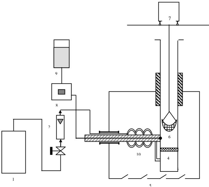
**Fig.2 Experimental apparatus for TG-analysis.**
