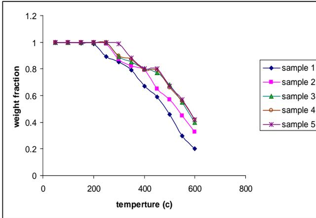
Fig.6 TG – analysis for matrices system RPU-M-F.
