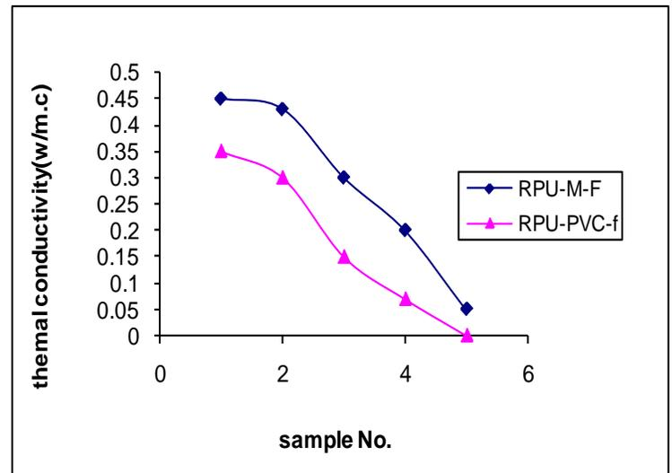
**Fig.5 Effect of promoter additives on the thermal properties of RPU.**
