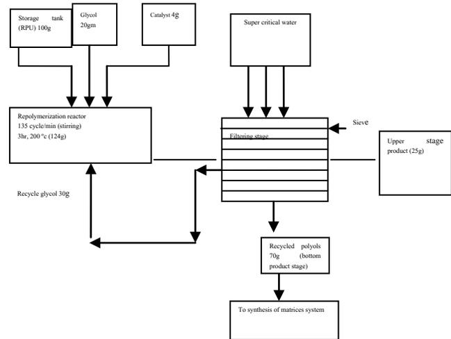
**Fig.1 Schematic blocking diagram for repolymerizing RPU scrap foam**
