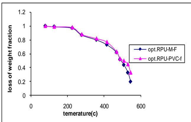
Fig.8 a comparison between TG – curves of two matrices system (RPU-M-F, RPU-PVC-f).
