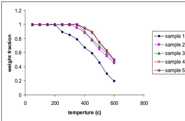
Fig.7 TG – analysis for matrices system RPU-PVC-f.
