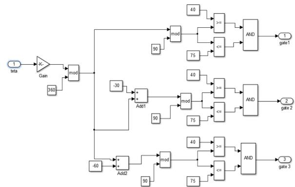
Fig. 9 Simulink model of theta position sensing
