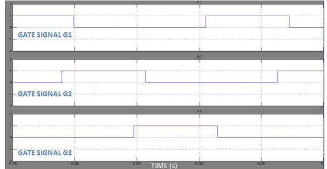
Fig. 7 Gate signals for the asymmetric converter
