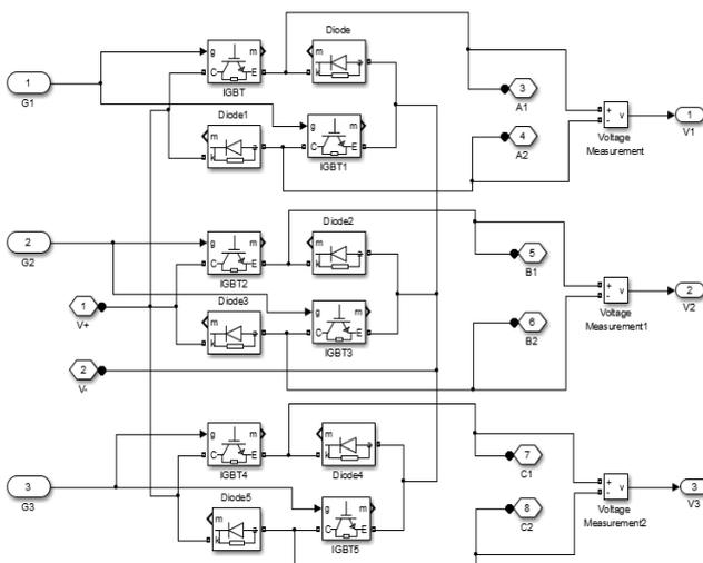
Fig. 6. Simulink model of Asymmetric converter
