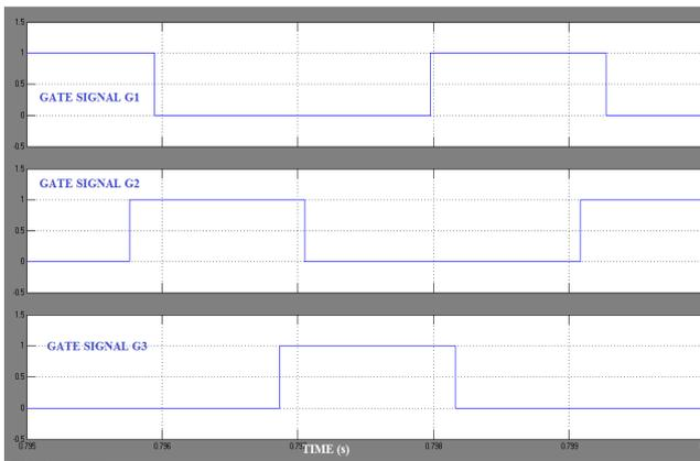
Fig. 11 Gate signals generated through theta position sensing
