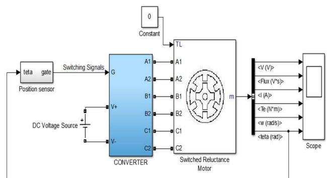
Fig. 5 Simulink model of open loop control of SRM
