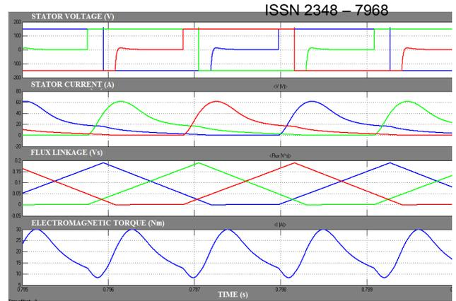
Fig. 12 Motor output waveforms of open loop control
