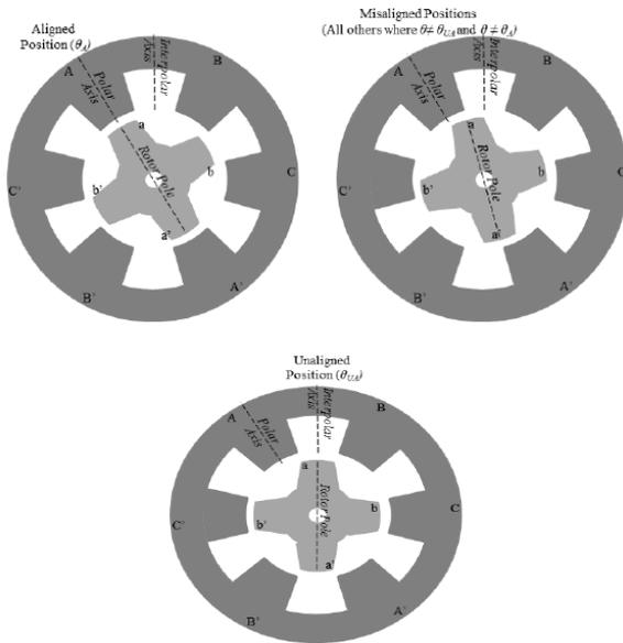
Fig. 2 Misaligned, aligned and unaligned positions for SRM
