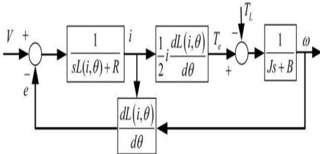
Fig. 4 Block diagram of single phase of SRM
