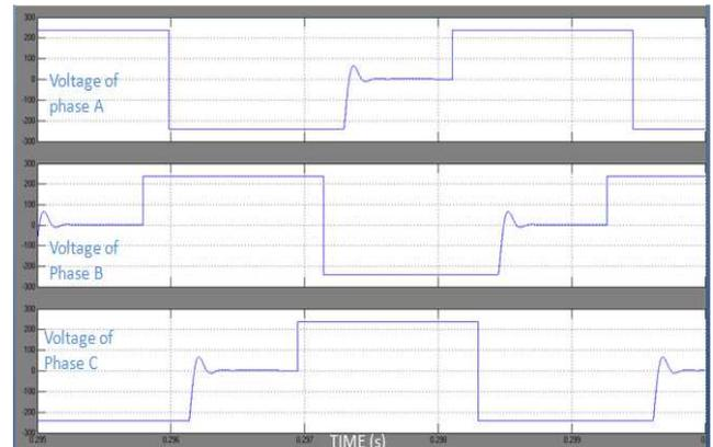
Fig. 8 Output voltage waveforms of asymmetric converter
