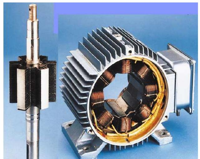
Fig.1. Stator and rotor of switched reluctance motor
