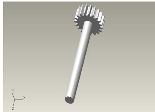
Figure 3. Pinion gear
