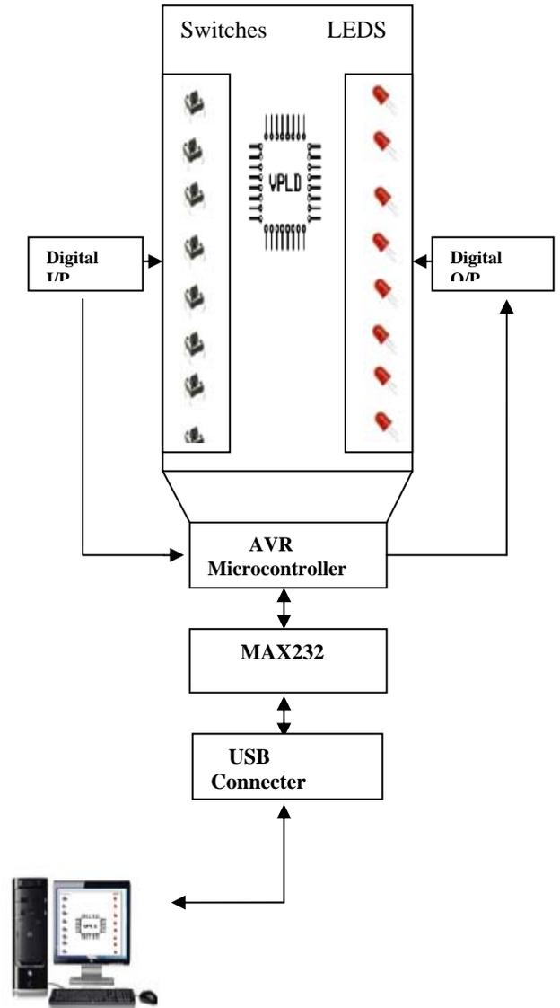
Fig.1 Block Diagram
