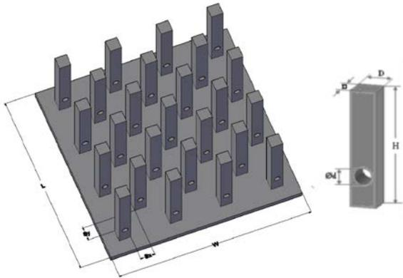
Fig. 2 Base plate having  $S_y/D=1.208$ . No. of fins 25.
