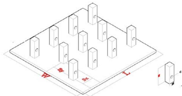
Fig. 1 Base Plate with Square fins in staggered arrangement.
